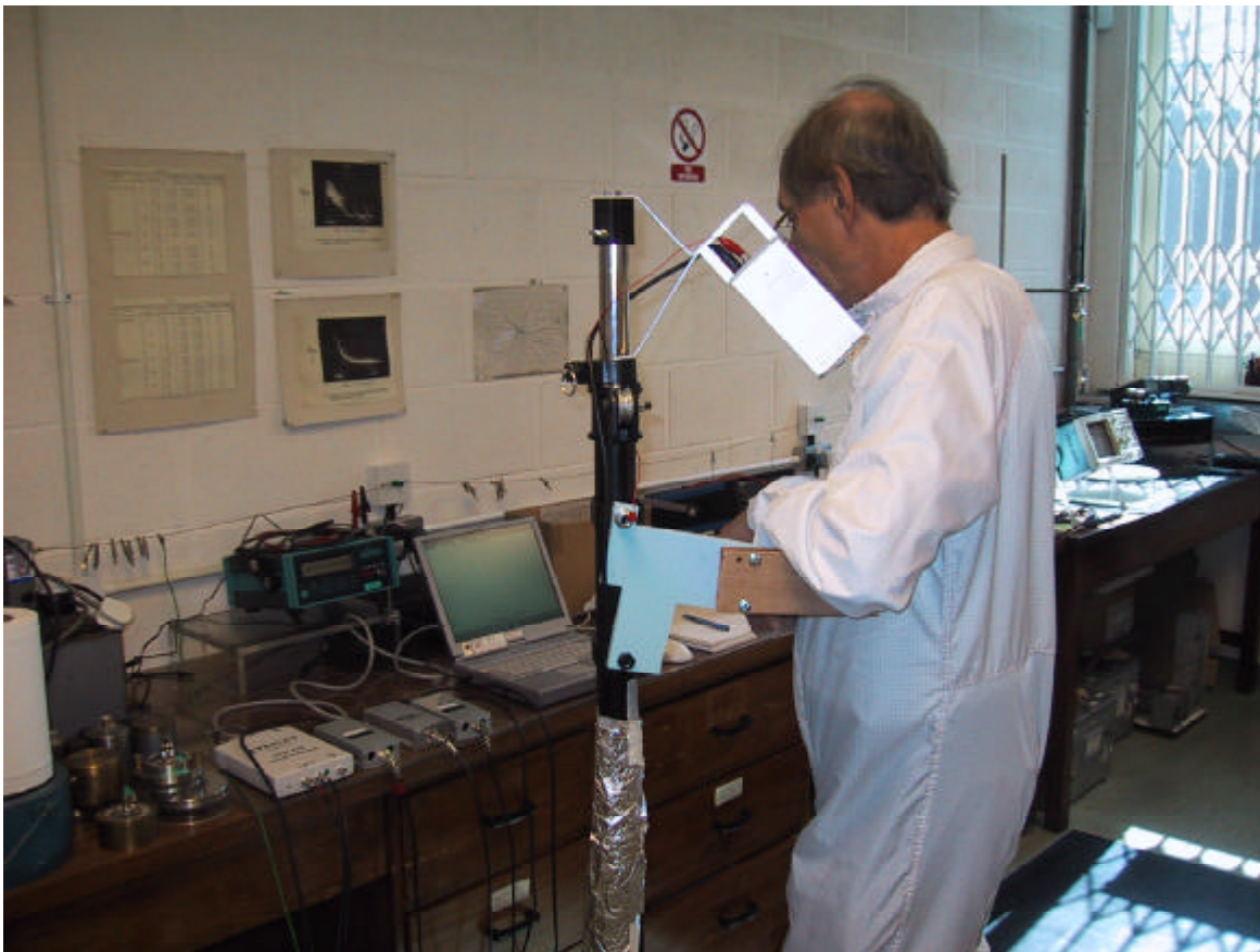
Figure 1: Operator in cleanroom garment with arm steadied on insulated rest from tripod support.
