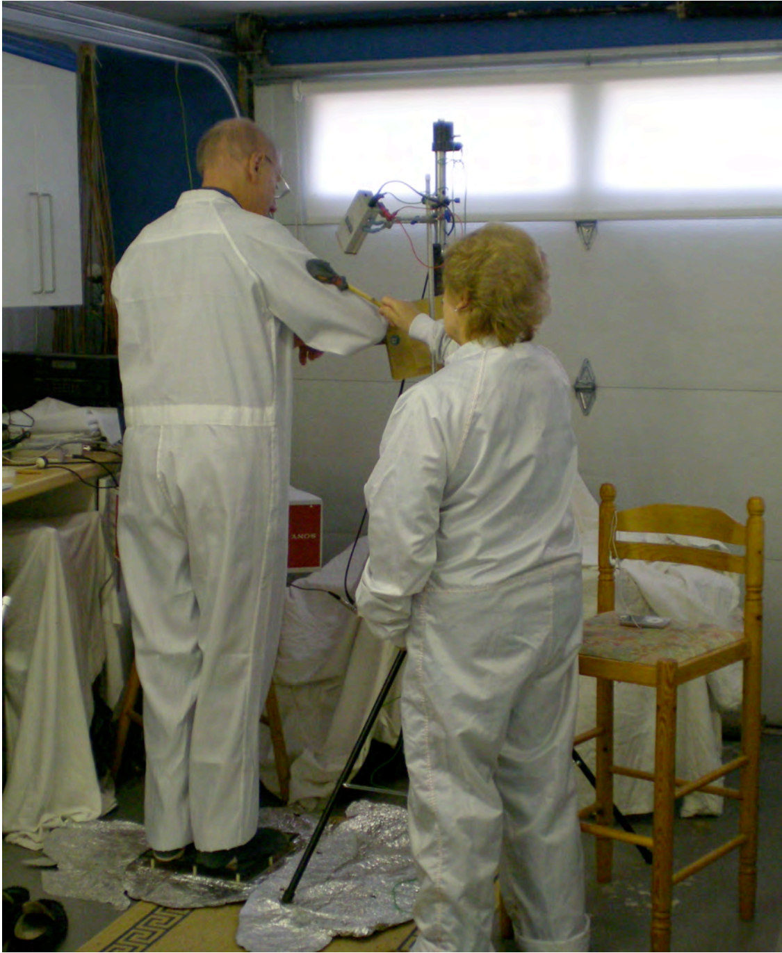
Figure 1: Set-up for testing inhabited garments. Test subject standing on charge measurement plate with arm supported on insulated support. Test operator ready to tribocharge area of sleeve directly in front of the fieldmeter.
